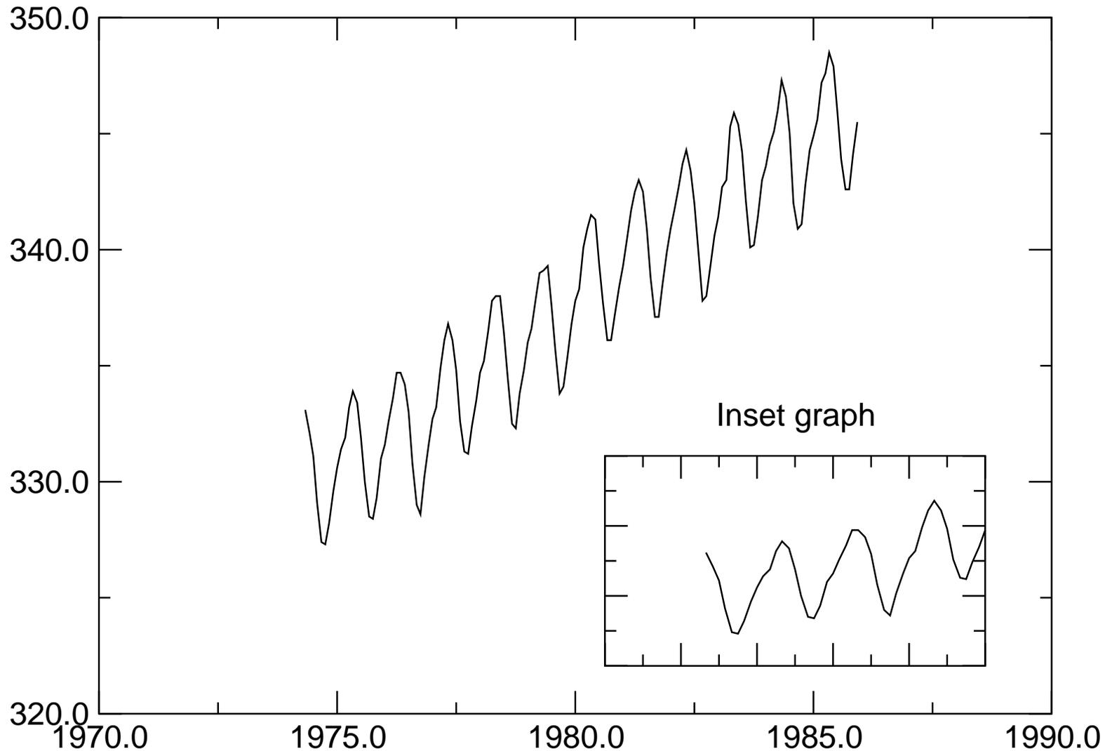
To make a graph within a graph, simply activate a graph and set the viewport to the desired location. Some problems may arise with getting/setting the graph focus, use the popup menu of any graph selector (e.g. in Plot/Graph appearance) to set the focus to a particular graph.
