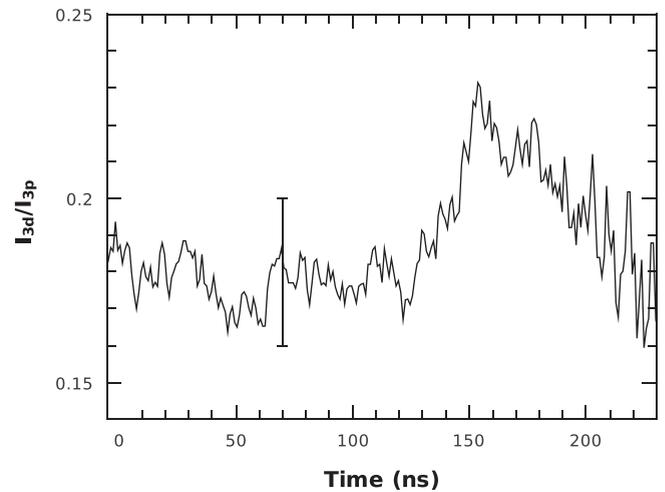
FIG. 2. Evolution of the line intensity ratio  $I_{3d}/I_{3p}$  measured at  $z = 37 \text{ mm}$ . The term  $Time = 0$  represents the beginning of the current-pulse.
