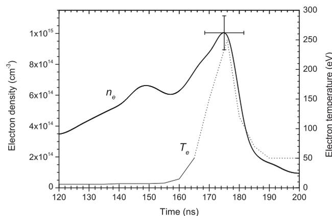
FIG. 7. The inferred evolution of  $n_e$  and  $T_e$ . For  $t \geq 165$  ns,  $T_e$  is only an estimate (marked by the dotted curve), but has no significant effect on the present B II-III modelling. The error bars reflect only the errors due to the uncertainties in the initial  $n_e$  and  $T_e$ , and not the uncertainty in the B II/B III ratio.
