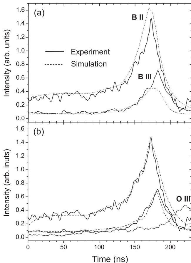
FIG. 6. Observed and simulated evolutions of the B II (3451 Å) and B III (2066 Å) intensities. (a) Initial parameters assumed are  $T_e = 4.5$  eV,  $n_e = 3.2 \times 10^{14}$  cm $^{-3}$ , and 10% B III. (b) The optimal fit found for the observation. Initial parameters assumed are  $T_e = 6.5$  eV,  $n_e = 2.1 \times 10^{14}$  cm $^{-3}$ , and 20% B III. Also presented is the intensity of O III transition (with an upper level of unit 49 eV), observed simultaneously with the B II transition.
