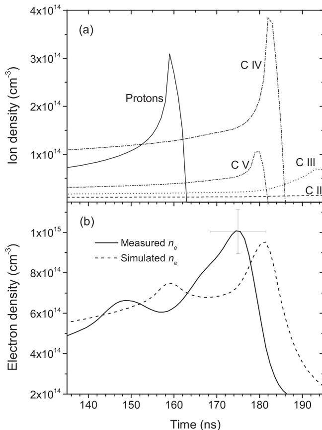
FIG. 9. (a) The simulated density evolution of the various ion-species based on the measured B II velocity and the assumption of a potential hill (see the Appendix) and (b) the resulting electron density evolution (convolved with the finite temporal response of the spectroscopic system), compared with the measured electron density.
