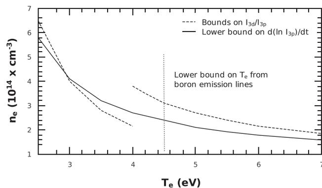
FIG. 4. Electron densities and temperatures that satisfy the lower and upper bounds of the intensity ratio  $I_{3d}/I_{3p}$  and the lower bound of the normalized Mg II ionization rate. The region above the solid curve and below the upper dashed curve corresponds to allowable  $n_e$  and  $T_e$  at  $t = 65$  ns (which is  $\sim 65$  ns prior to the magnetic-field arrival to the point of observation).
