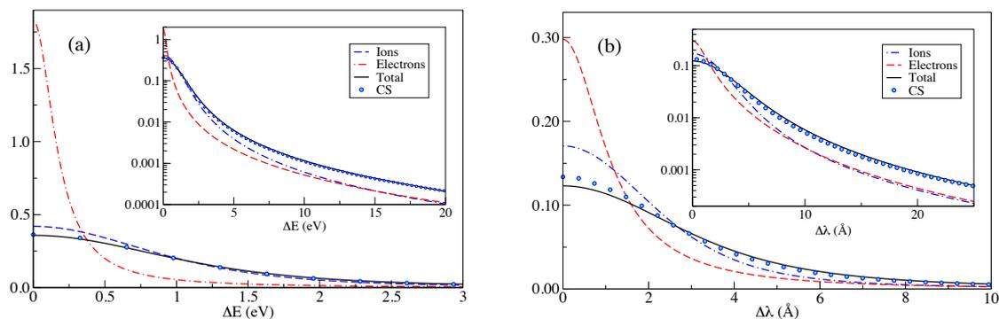
**FIGURE 3.** Comparison between analytical and computer simulation (CS) results of Stark broadening of a) Ne X Ly $\delta$  in deuterium plasma with  $N_e = 10^{21} \text{ cm}^{-3}$  and  $kT = 1 \text{ keV}$ ; b) D Balmer  $n = 9$  line in deuterium plasma with  $N_e = 5 \times 10^{14} \text{ cm}^{-3}$  and  $kT = 4 \text{ eV}$ .
