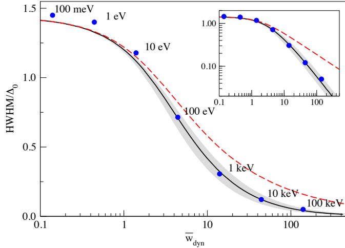
**FIGURE 2.** HWHM of the Stark broadening of H Ly $\delta$  due to proton perturbers with  $N_p = 10^{14} \text{ cm}^{-3}$ . Debye screening is neglected. -- calculations according to Eq. (22); — calculations according to Eqs. (27) and (29) with  $\bar{v}_0 = 5$ , with the hashed area indicating results obtained by varying  $\bar{v}_0$  between 2.5 and 10; • computer simulation results, annotated with the plasma temperature assumed.
