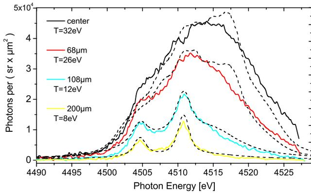
FIG. 3. (Color online) Comparison of assorted Abel-inverted experimental spectra (solid lines) from irradiation of a 10  $\mu\text{m}$  Ti foil and the best-fit modeled spectra (dashed lines).
