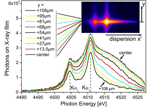
FIG. 2. (Color online) Single-pulse x-ray spectra of the laser-irradiated 10- $\mu\text{m}$ -thick Ti foil at laser intensity  $I = 5 \times 10^{19}$  W/cm<sup>2</sup> and  $\lambda = 1057$  nm, shown from different target positions  $y$ . The x-ray film scan (false colors) is given in the inset.
