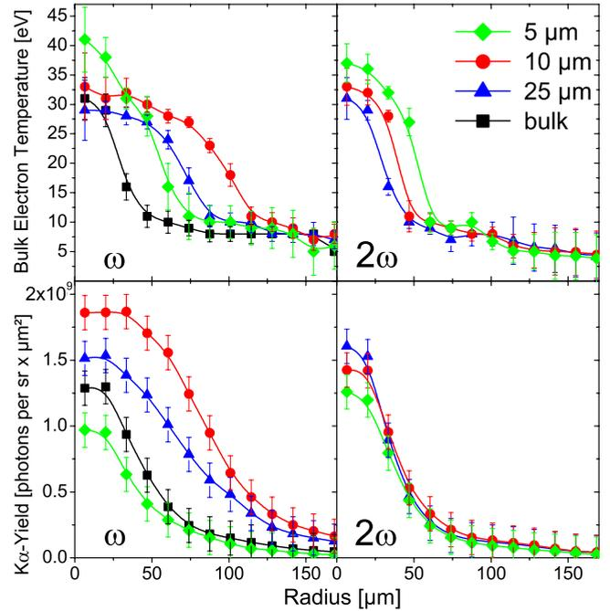
FIG. 4. (Color online) Radial temperature (top) and integrated  $K\alpha$ -yield (bottom) distributions of the different targets used, irradiated with the  $\omega$  and  $2\omega$  laser pulses.
