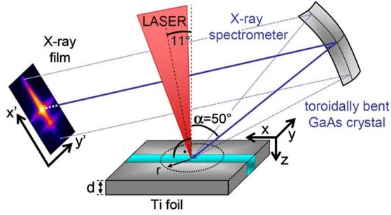
FIG. 1. (Color online) Schematic of the experimental setup. The energy dispersion axis  $x'$  on the x-ray film is perpendicular to the spatial resolution in the  $y$  direction.
