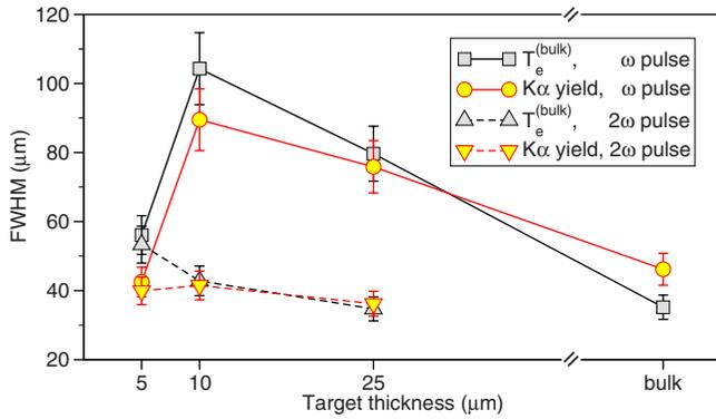
FIG. 5. (Color online) Comparison of FWHM of the bulk-electron temperature and  $K\alpha$ -yield radial distributions for different targets and laser pulses.
